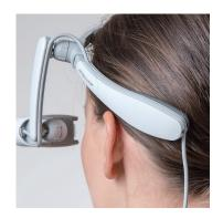
The newly designed headband and its flexible arm ensures that the AiRScouter WD-200B attaches to the user comfortably and securely for uninterrupted performance.
